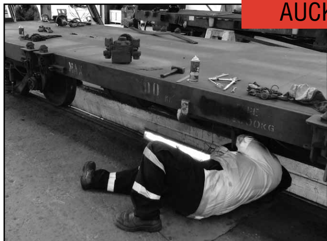
... repairing braking components on a bogie (above) and repairing the well-used points in the Westfield yard (right).
