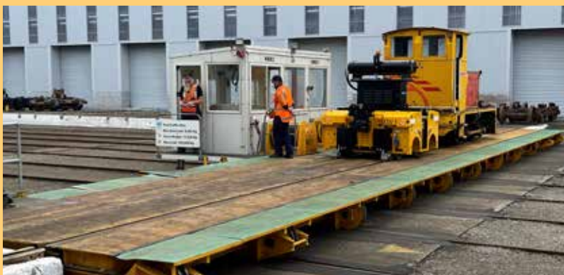
New and old shunts on the workshop traverser.
