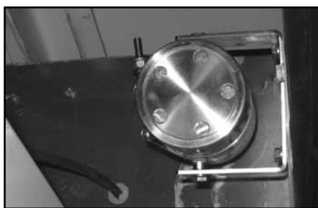
One of the STAT.X fire suppression canisters mounted in place. This one is on one of the Tranz Alpine AKV vans.
