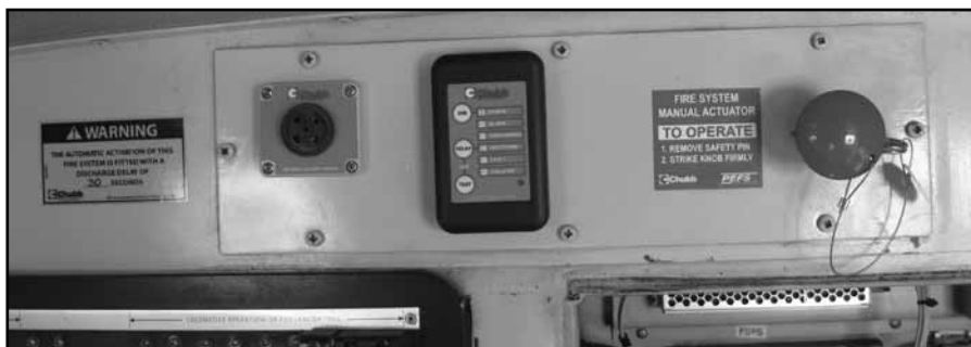
The Chubb STAT.X control panel on the cab rear wall of DXC5477.
