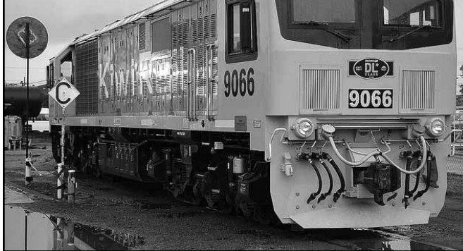
A typical asbestos-laden Chinese-built DL loco.
